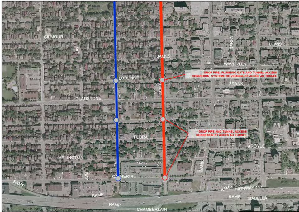
Figure 4: Site 3 Kent at Catherine; site plan of the Project Area showing the preferred alignment and proposed tunnel accesses.
